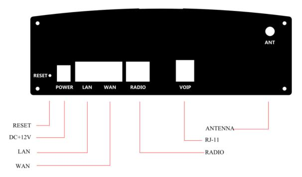
**ANT**: When the radio is built-in, VHF/UHF antenna can be setup.
